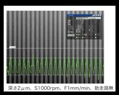
fabrication test, 2µm pitch
