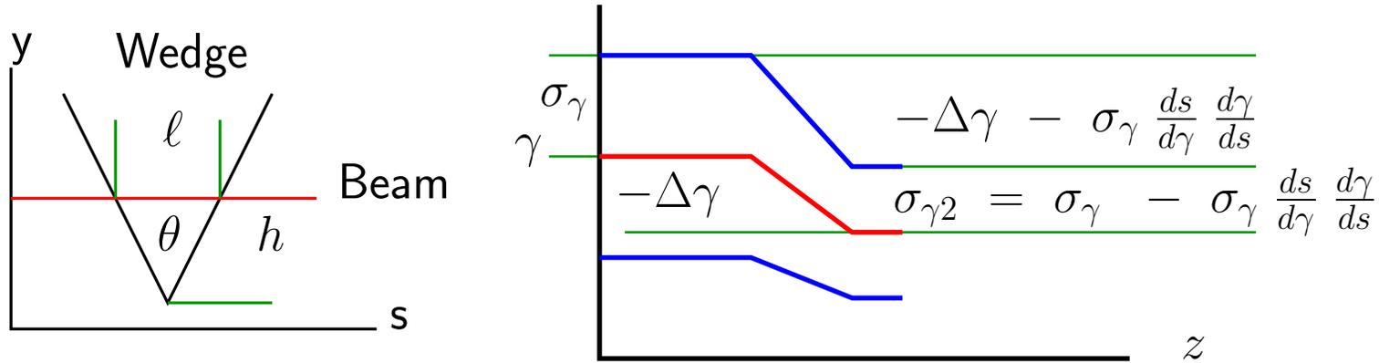
For a wedge with center thickness  $\ell$  and height from center  $h$  ( $2h \tan(\theta/2) = \ell$ ), in dispersion  $D$  ( $D = \frac{dy}{dp/p} : D = \beta_v^2 \frac{dy}{d\gamma/\gamma}$ ) (see fig. above):
