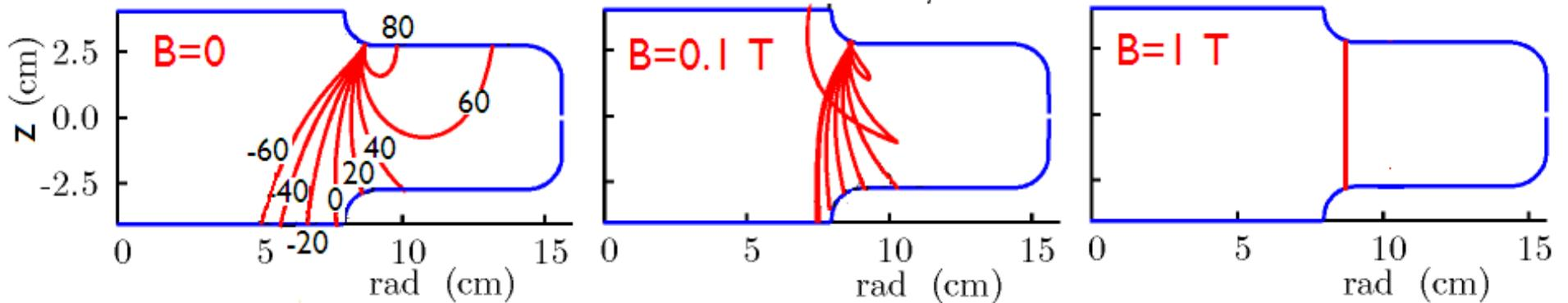
1. "Dark Current" electrons accelerated and focused by magnetic field
