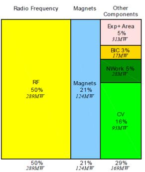
CV: cooling & ventilation, NW: electrical network losses, BIC: beam instrumentation & control
