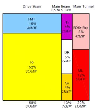
RF: drive beam linac, FMT: frequency multiplication & transport, So: sources & acceleration up to 2.5 GeV, DR: damping rings, Tr: booster linac up to 9 GeV & transport, ML: main linacs, BDS: beam delivery system, main dump & experimental area
