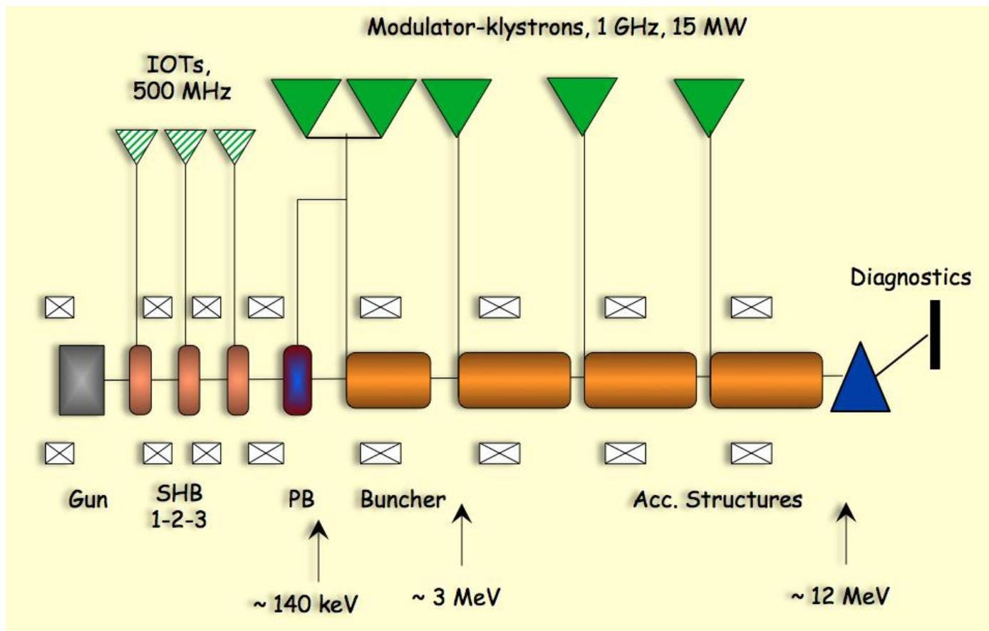
Gun, sub-harmonic bunching, bunching, three accelerating structures,
