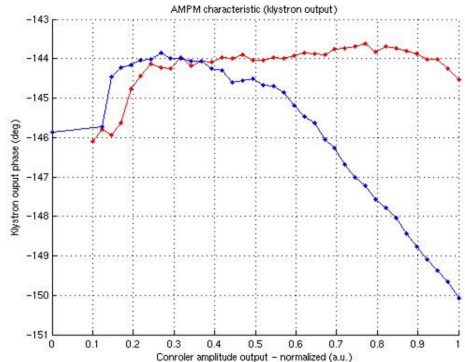
Proposed and implemented method allowed for klystron behavior linearization. Although some system weak points can be recognize (eq. poor phase detection for low signal levels) amplitude and phase characteristic correction can be considered as satisfactory.
