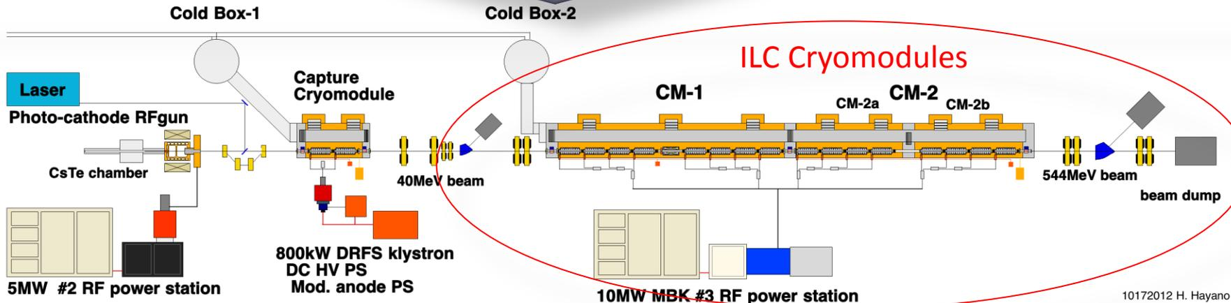
1ms bunch train with 2.5mA beam are successfully accelerated to 40MeV in Injector operation, 4 mirror laser accumulator is ready for X-ray generation experiment.
