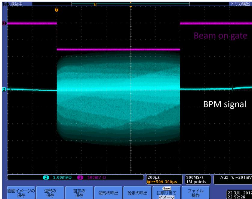
1ms flat Beam extraction from RF-gun 1ms
