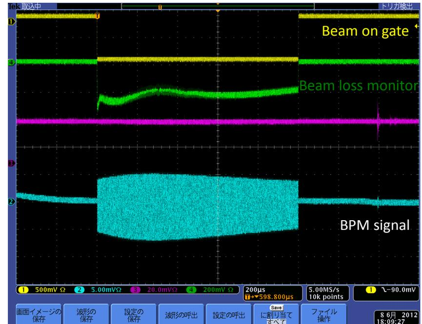
Beam acceleration with 1ms train (15pC/bunch)
