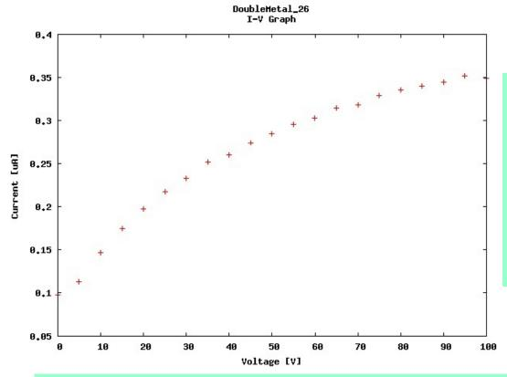
SiD Leakage Current (sensor #26): Average leakage for 1840 channels is about ~160 pA/channel
