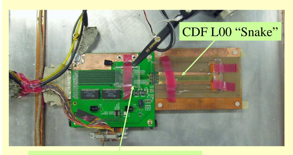
LSTFE1 chip on Readout Board
