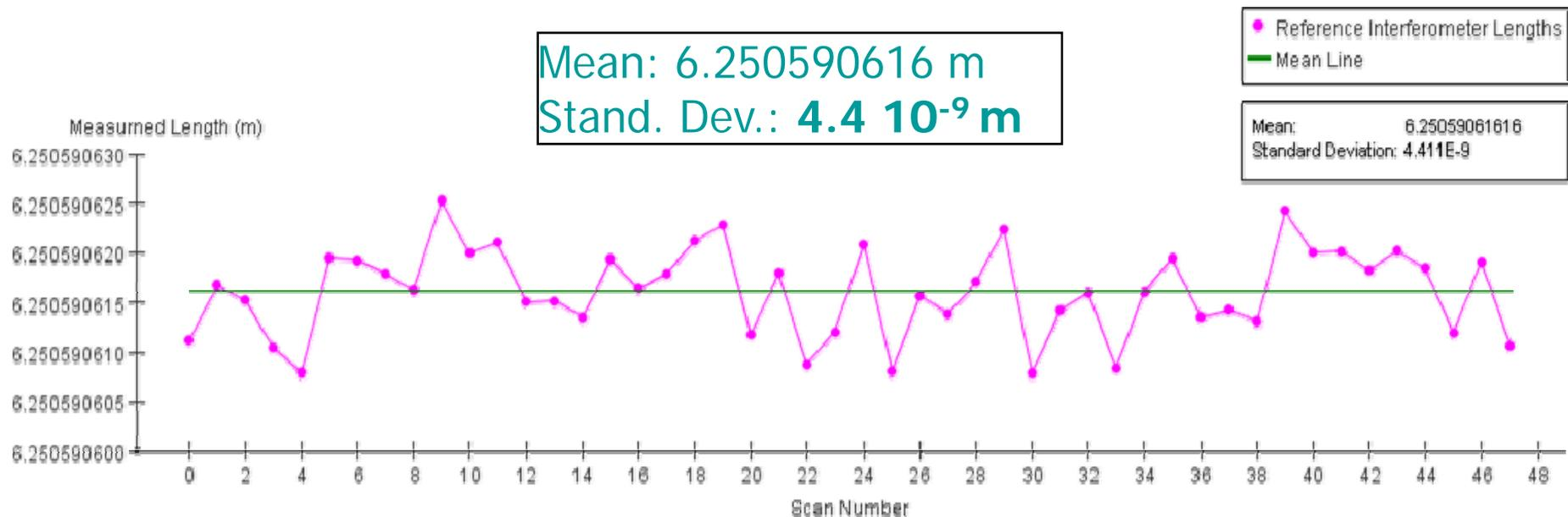
Fig. 2 Repeatability of FSI Ref. Interf. measurements
