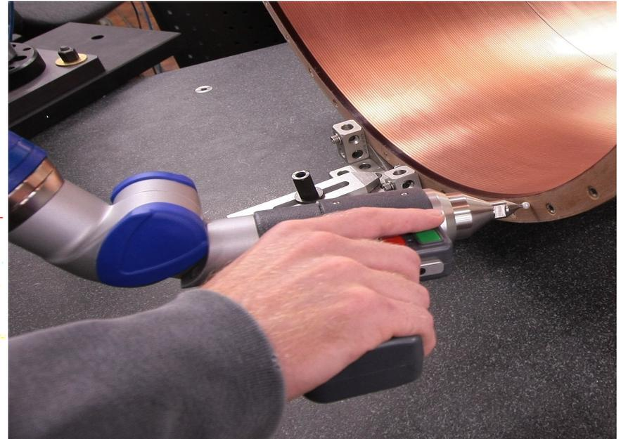
Intrinsic measurement precision per point: around 20  $\mu\text{m}$
