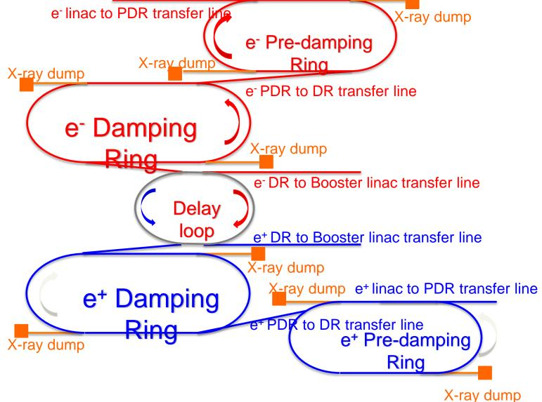
The modification is to allow injection to e+ pre-damping ring from a different direction
