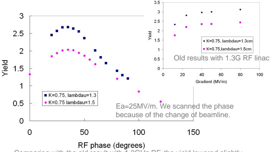
Comparing with the old result with 1.3GHz RF, the yield lowered slightly when using 2GHz RF.
