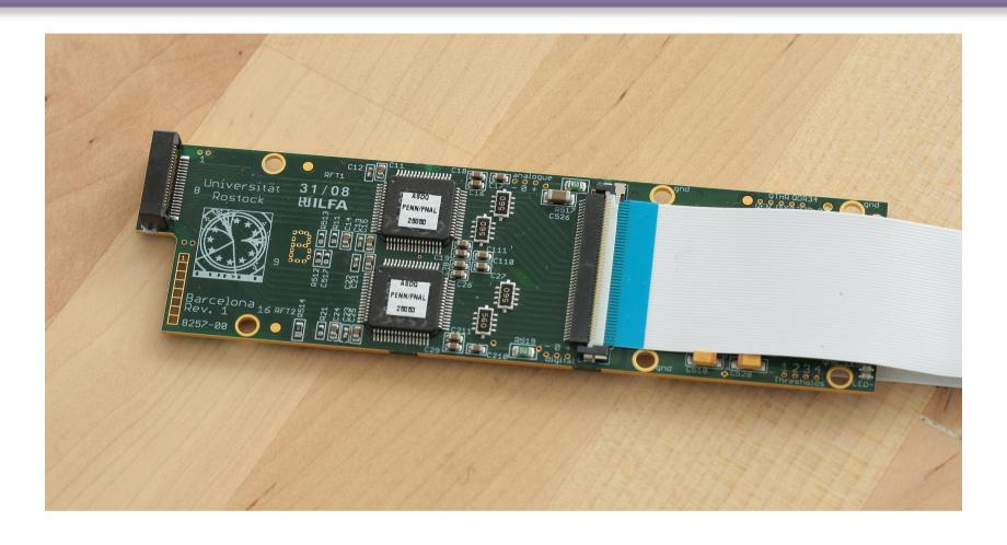
32 channels (4 ASDQ chips) in 30 mm \* 106 mm Top-to-bottom thickness: 4.4 mm
