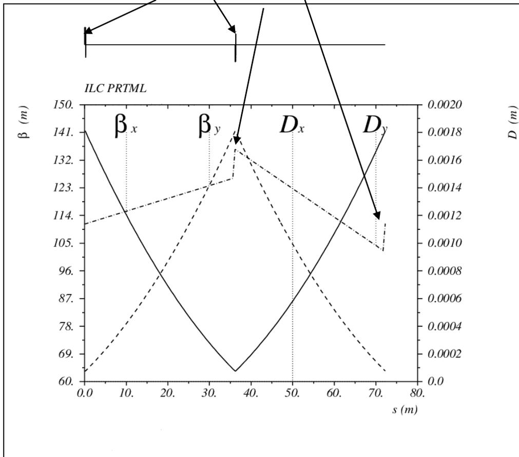
Geometric curvature of the beamlines is realized in the vacuum chamber and the beam orbit is curved by means of vertical dipole correctors at each quadrupole of the FODO lattice. A small vertical dispersion is then created and propagated along the line. The first 4 correctors and the last 4 correctors are used to match the curved section to the straight lines.
