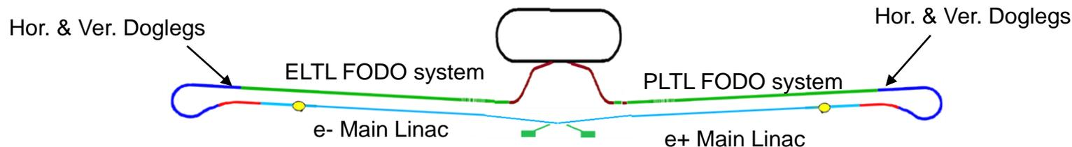
For Cryogenic requirements main linacs need to follow the curvature of the Earth.
