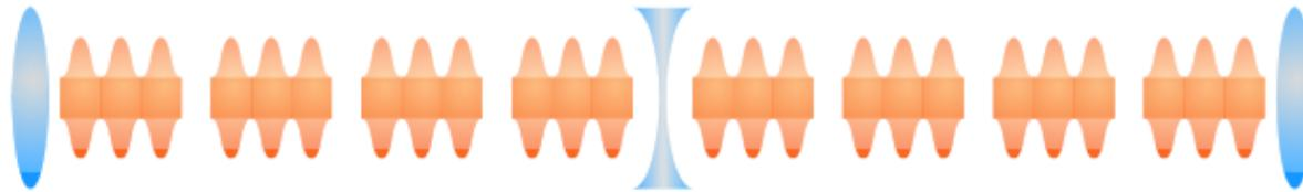
6140 MV integrated voltage, 2 GHz frequency, 15 MV/m gradient, 410 m of cavities, 1.5 m cavity length, 274 cavities embedded in a FODO lattice with 8 cavities per cell, total length 472 m.
