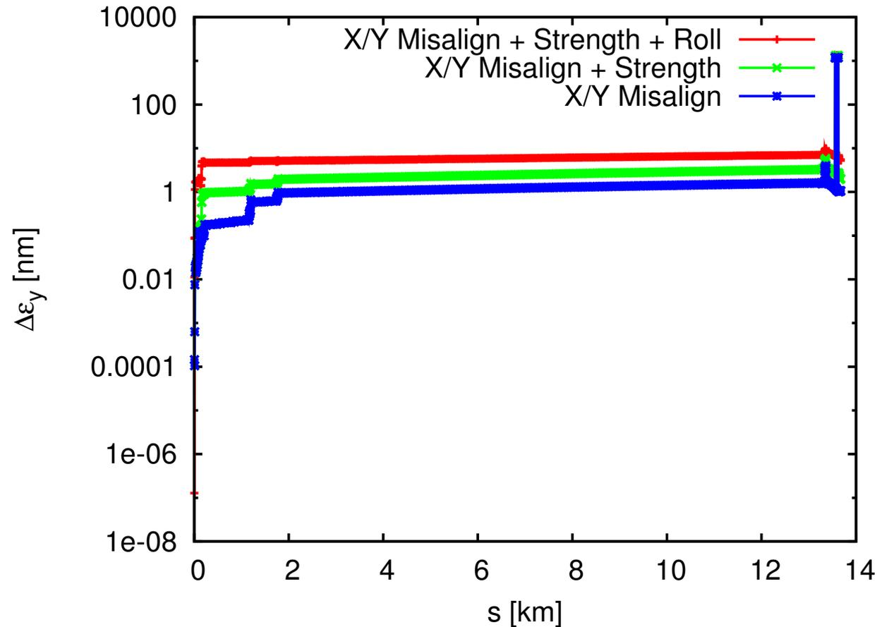
⇒ X/Y Offsets: Final average emittance growth is 1.06 nm (1.58 nm 90% c.l.)
