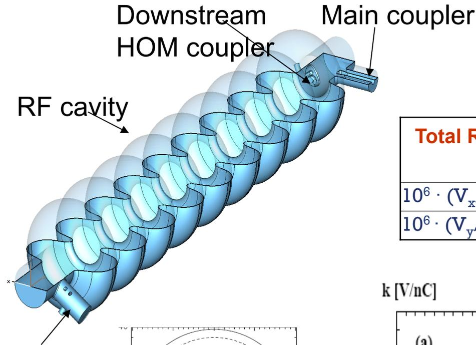
The couplers break the RF field symmetry and cause transverse RF kick and Wakes
