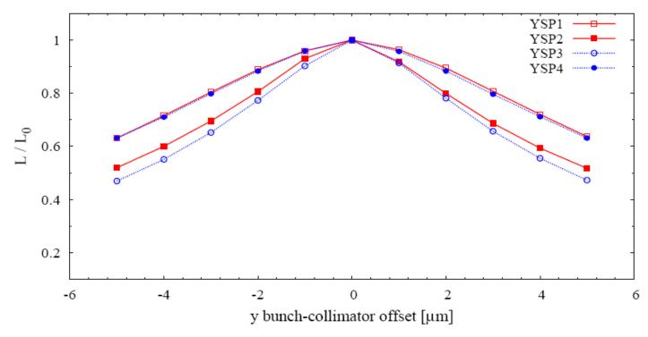
Collimator misalignment tolerance  $1/2 \sigma_y \approx 1 \ \mu m \ (\sim 10\% \ luminosity \ loss)$  (one order of magnitude smaller than ILC tolerance)
