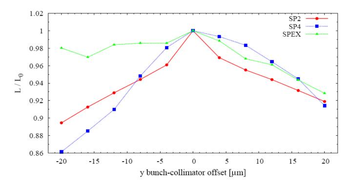
Collimator misalignment tolerance  $\approx 20~\mu m~$  (  $\sim 10\%$  luminosity loss) It can be achieved with optical survey alignment techniques!
