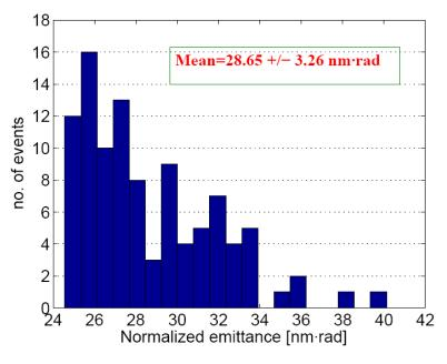
Vertical emittance dilution for 100 seeds of applying misalignments (static and GM), 1-to-1 and DFS correction
