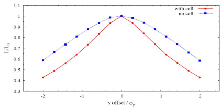
Jitter tolerance  $0.2 \sigma_y$  ( ~ 10% luminosity loss) (Similar to ILC initial jitter tolerance)
