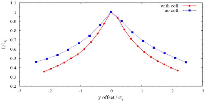
Jitter tolerance  $\approx 0.2~\sigma_v^{}=0.4~\mu m$  ( ~ 10% luminosity loss)
