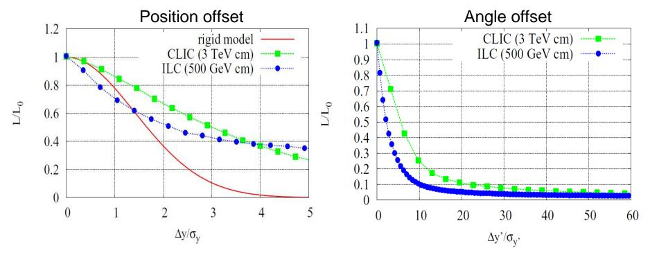
Simulations with Guinea-Pig: beam-beam effects (beamstrahlung, hourglass effect, pair creation, ...). Disruption parameters:  $D_y$ =19.4 (ILC);  $D_y$ =3.5 (CLIC)
