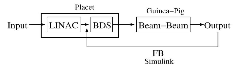
For the ILC we use a proportional and integral (PI) controller algorithm embedded in Simulink (MATLAB)
