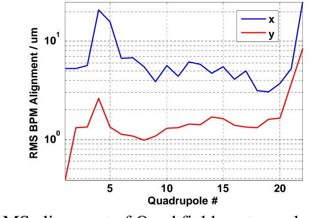
RMS alignment of Quad field center – electrical center of Quad BPMs (100 seeds).
