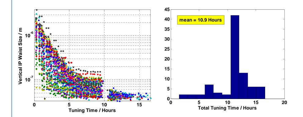
□ Multi-knobs iteratively applied until IP beamsize growth over initial conditions is <10% (~<40nm).
