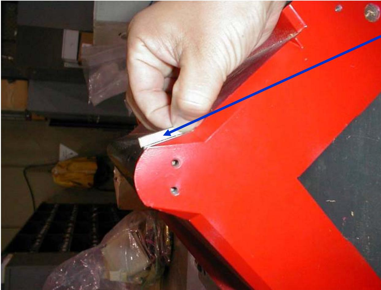
Width of shim carefully chosen so does not interfere with adjacent coil [which vary a little in size from
