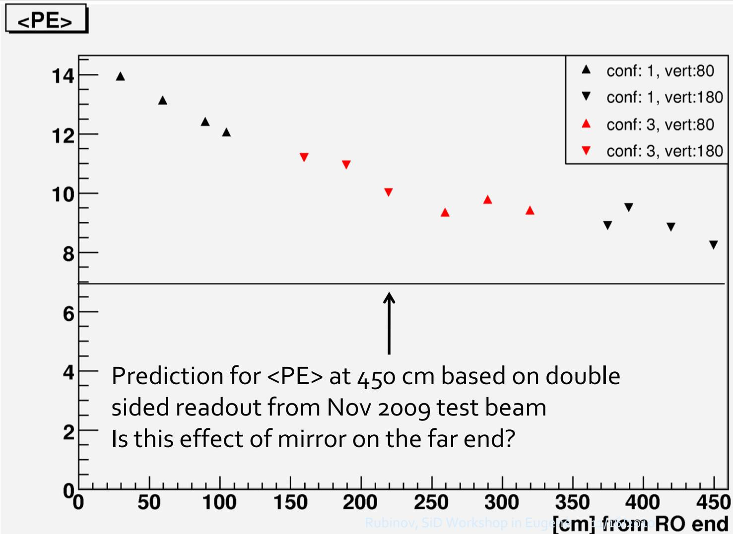
The signal fraction "S" as a function of distance "d" from the sensor is  $S(d)=\exp(-d/L_{\text{eff}})$  and  $L_{\text{eff}}= L_0+c*d$
