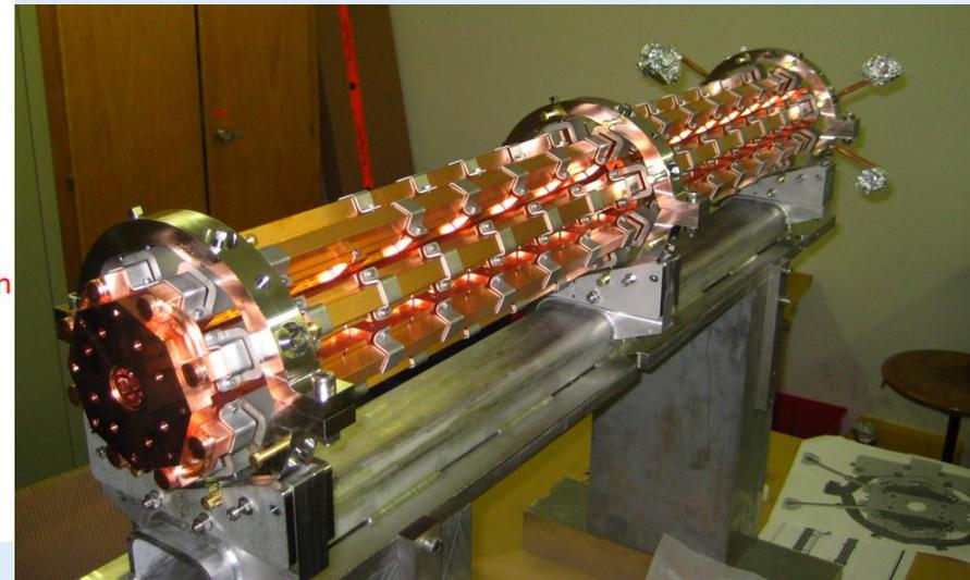
1500 x 48 power extraction and transfer structures (PETS) will convert kinetic energy to rf power along 1 km decelerator sectors.
