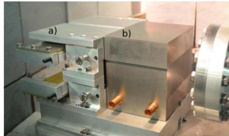
Figure 18: Picture of the segmented beam dump (a) installed in the beam line with a water-cooled collimator in front (b).
