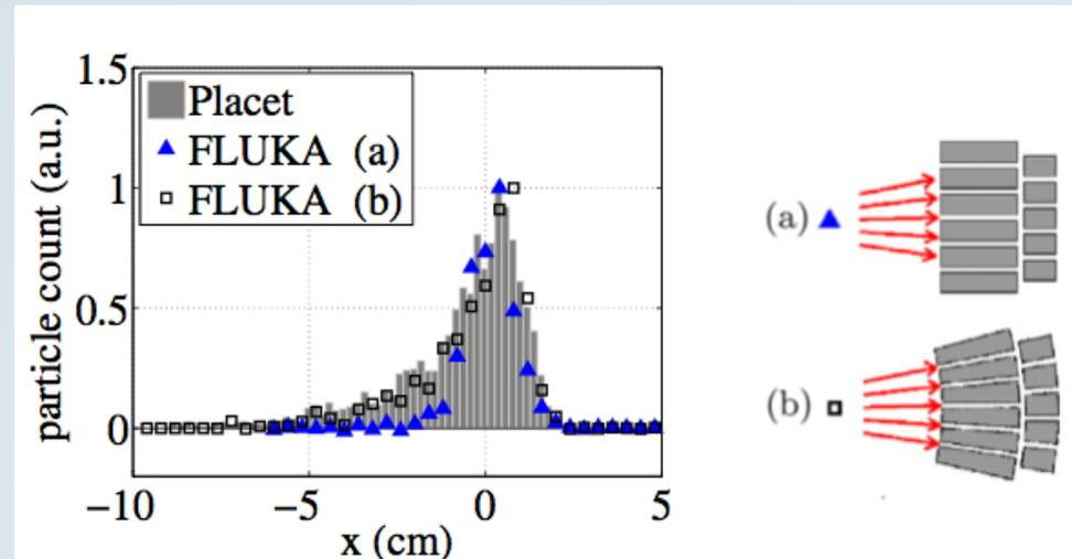
Concentric geometry of the segmented dump (b) ensures good resolution of the energy profile.
