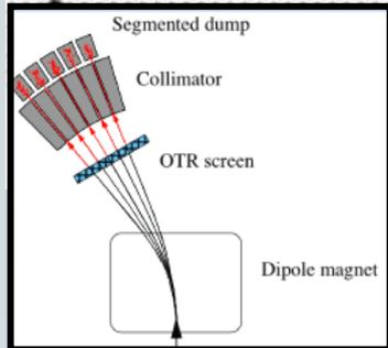
Optimized segmented dump for complete energy measurement (Uppsala U./CERN)
