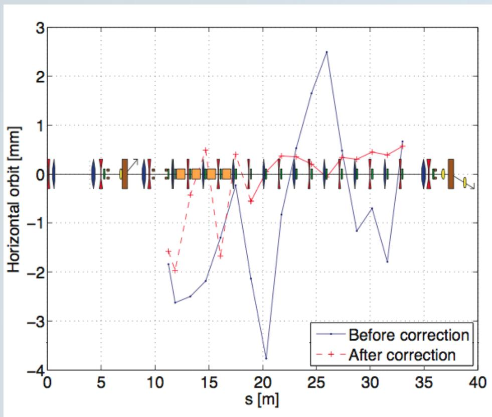
Automatic orbit control in TBL. 2013: plans to test dispersion-free steering schemes.
