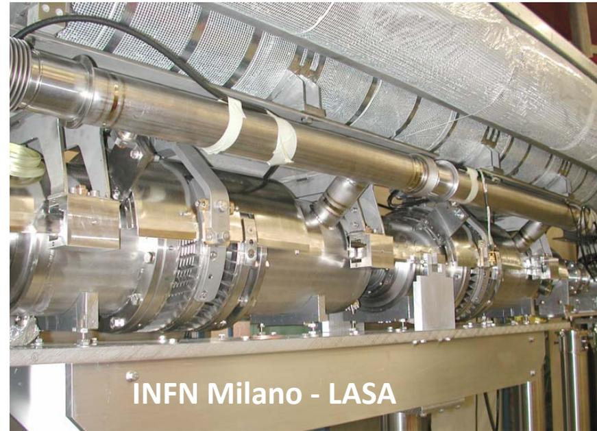
**Concept:** through thin “blades” transform the rotation of the 2 center ring halves in a longitudinal axial motion that changes the cavity frequency modifying its length.
