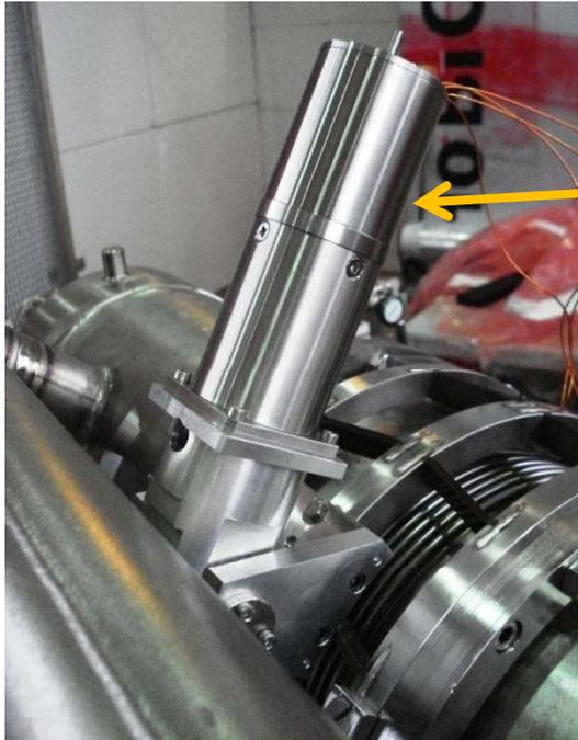
The same Blade Tuner assembly has been installed for cold testing at BESSY, except for the driving unit, a stepper motor equipped with **planetary gear**
