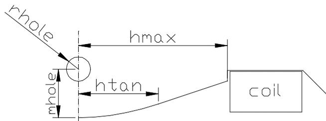
Iron pole parameters for 2-d magnetic optimization
