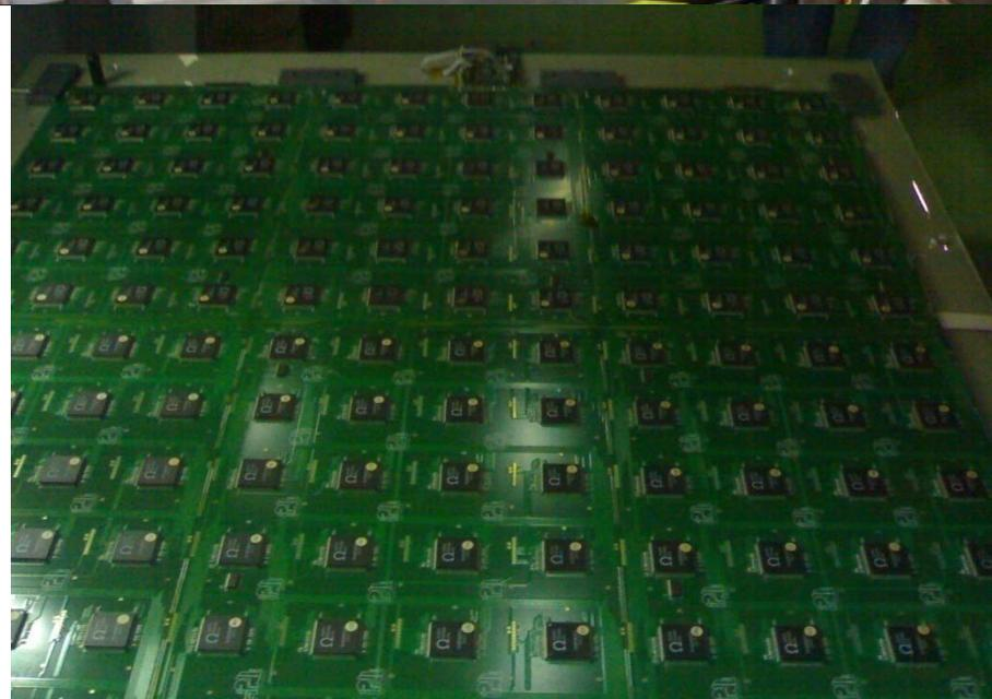
test of large area RPC & μMEGAS for SDGHcal in progress
