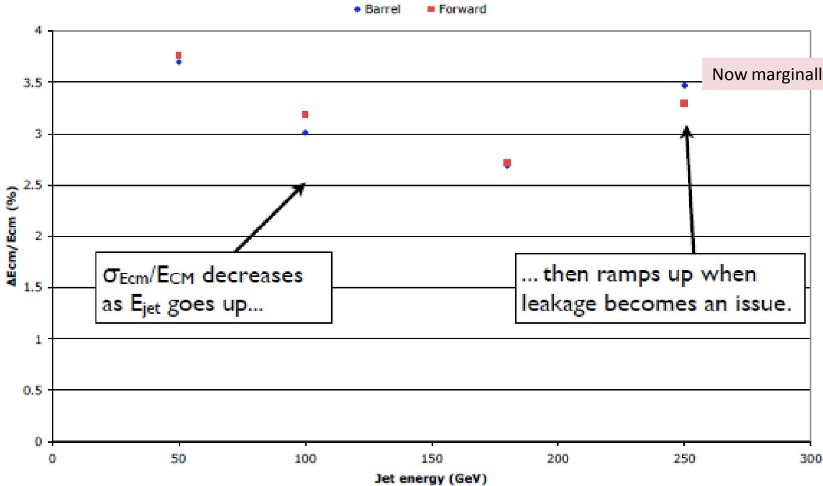
At higher energies resolution worsened partly due to leakage *but also due to algorithm*
