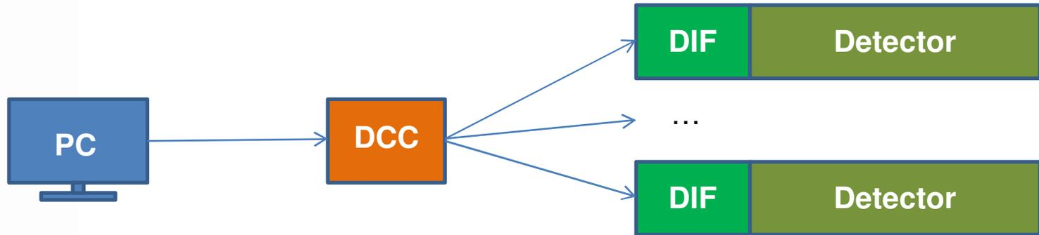
After debugging the code at LLR with the setup above (thanks to Rémi and Franck for their precious help), the DHCAL DIF is now working in the CALICE DAQ architecture.
