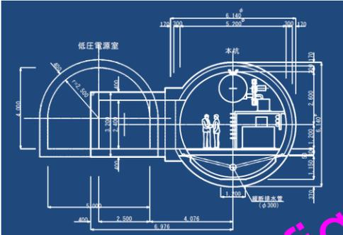
In each 152m, low voltage power facility (LVPF) is introduced and 6.6kV power is reduced to 420 V to deliver power to 4 stations.
