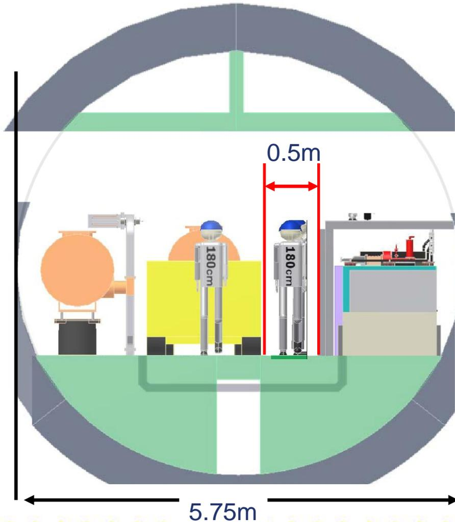
Another alternative plan is to increase the tunnel diameter from 5.2m to 5.75m.
