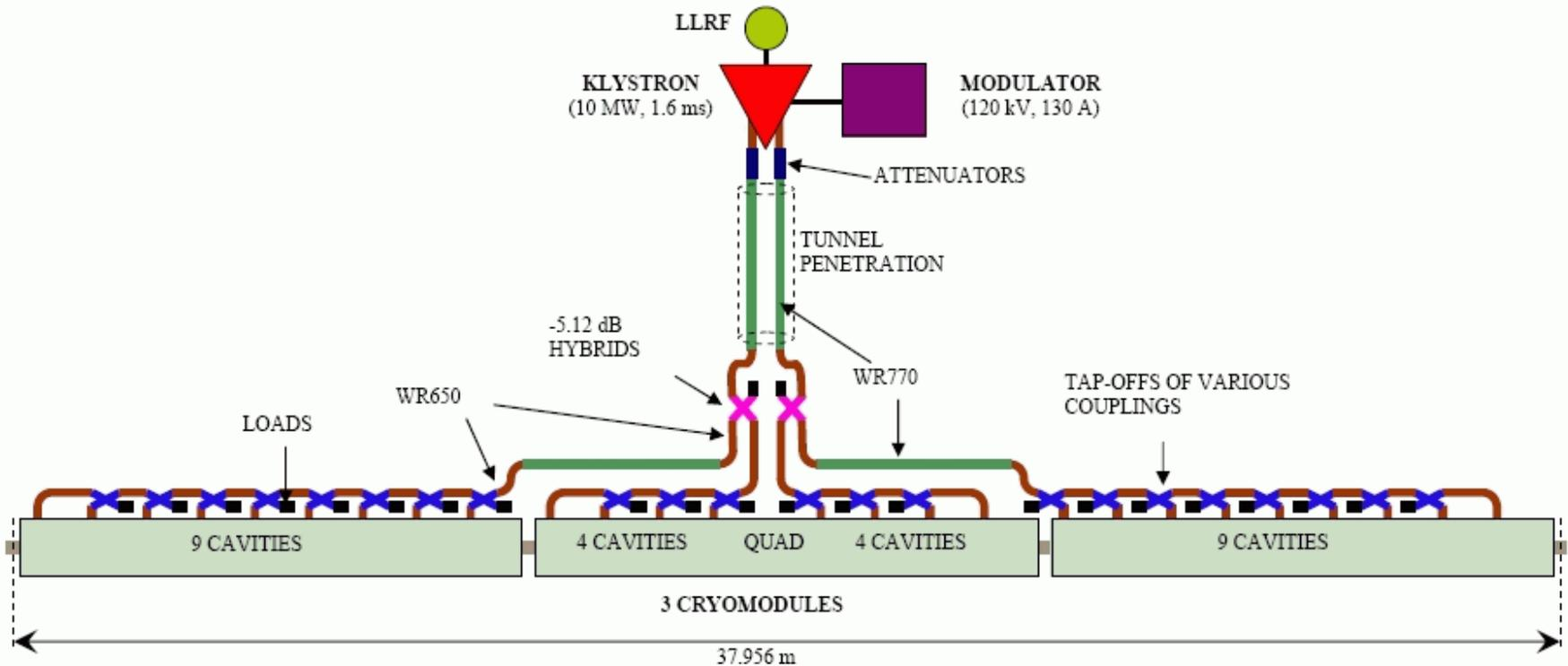
Positron linac uses 278 RF units to accelerate beam from 15 GeV to 250 GeV; electron linac uses 282 units (4 units make up energy loss in positron production process).
