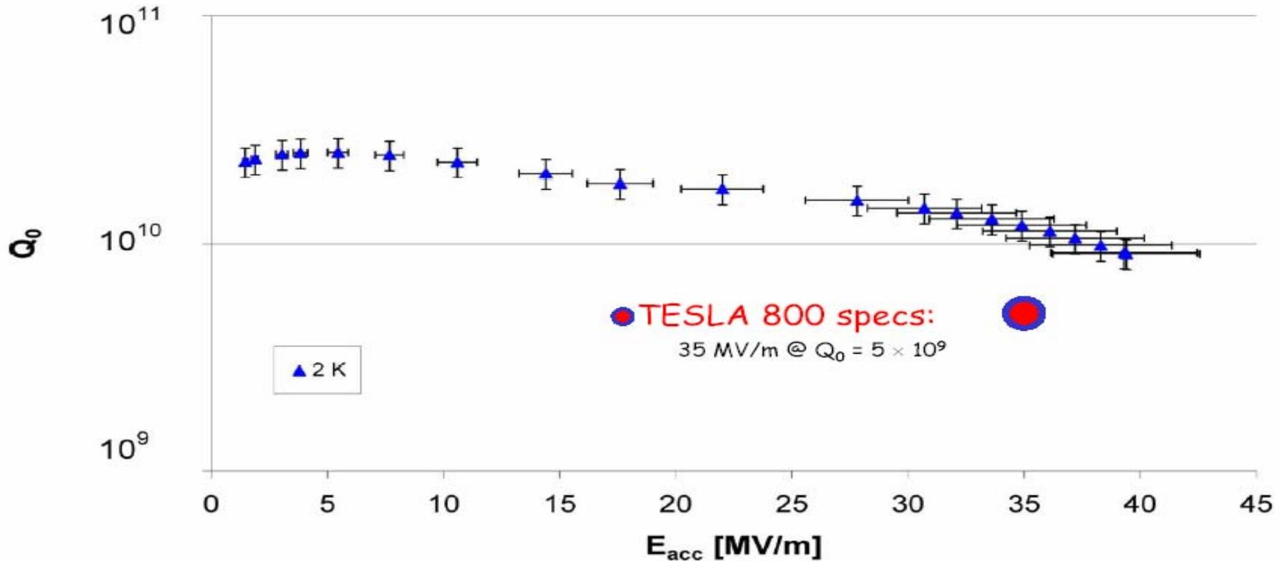
Operating accelerating gradient is a compromise between real estate bill (favors high gradient) and cooling bill (favors low gradient). Compromise = 31.5 MV/m. At 43 MV/m, magnetic field on cavity iris is ~"critical field", causing cavity to suddenly leave SC state ("quench").
