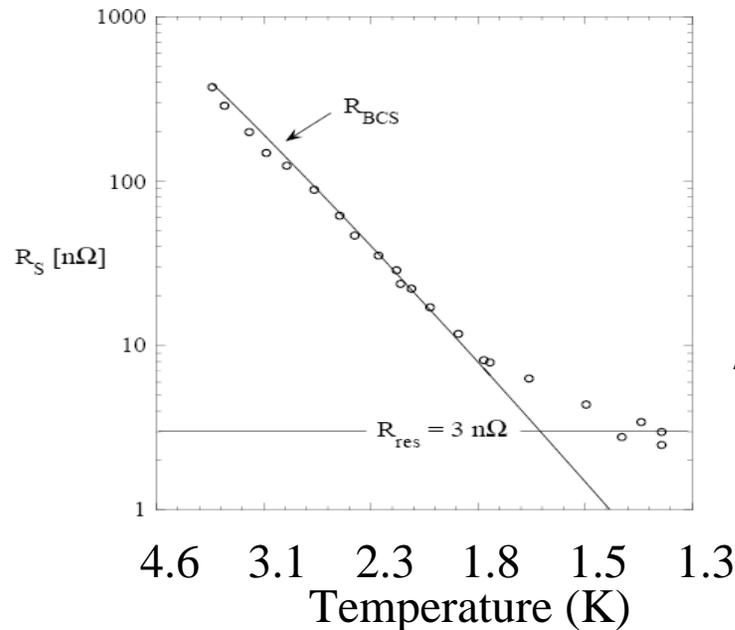
Operate at 2 K – below this level, resistance starts to be dominated by residual, rather than natural SC AC resistivity!
