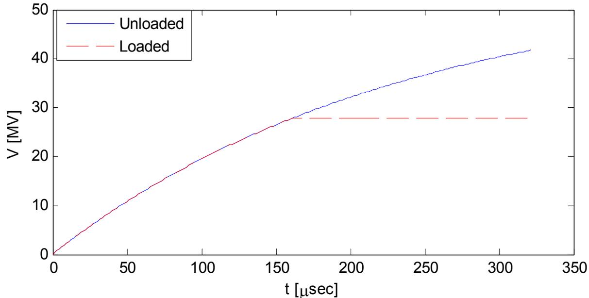
The fields induced by the beam in the unpowered cavity must be given by the difference between these two lines!
