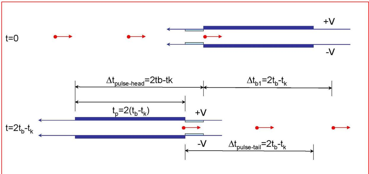
As shown in the sketch, the pulse must enter the kicker structure after bunch 1 exits the structure. Then the pulse must exit the structure before bunch 3 enters the structure. Using the relationships shown in the sketch above, the time between the leading and trailing edge of the pulse must satisfy the specified relationship.
