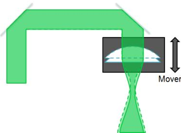
**Focal scanner → align focal point to IP**
