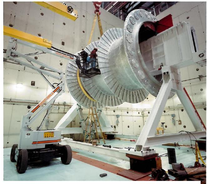
SLD, Liquid Argon Calorimeter
