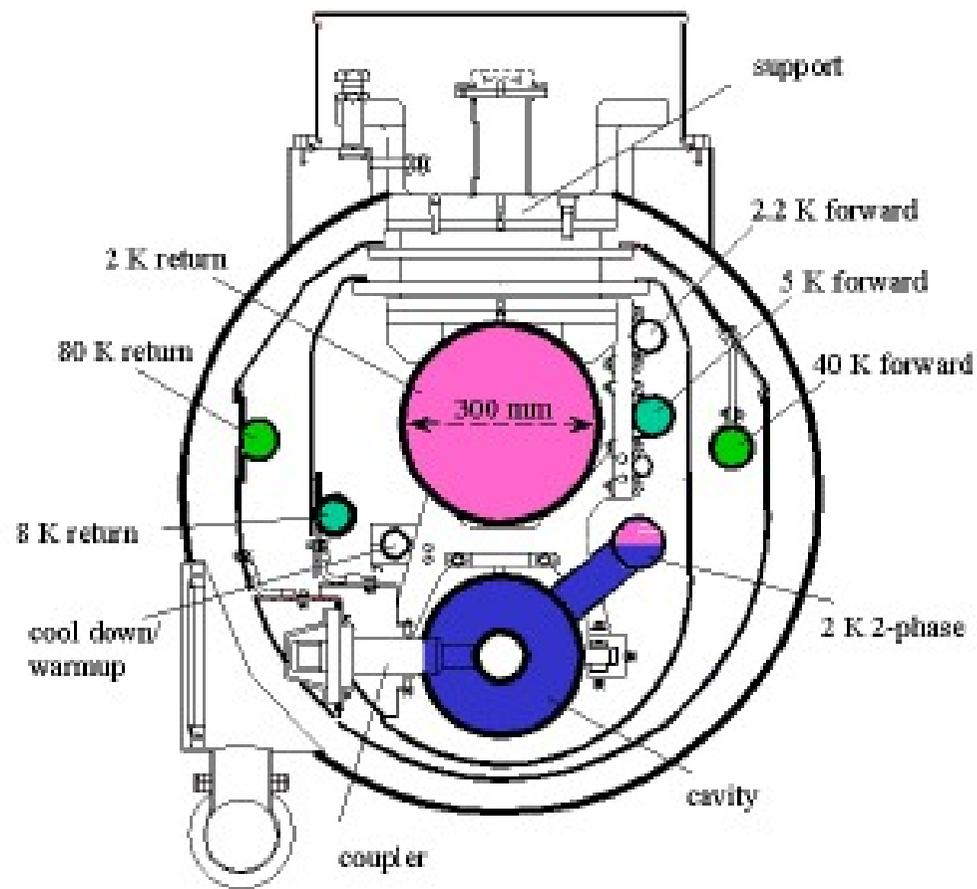
Figure 3.2.11: *Cross section of cryomodule.*
