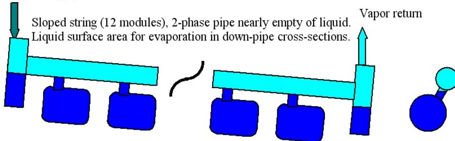
This is the way that a sloped ILC (and XFEL) would operate, with liquid running down the 2-phase pipe, filling each helium vessel, and excess liquid dropping into a vessel at the string end where it is boiled away by a small electric heater.
