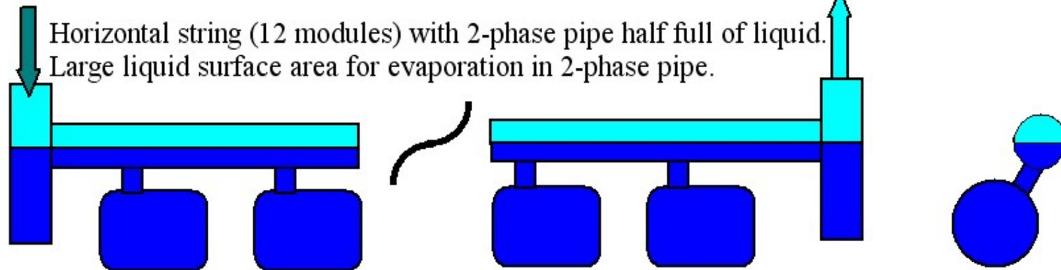
This is the way that TTF has been running, with liquid partially filling the 2-phase pipe.
