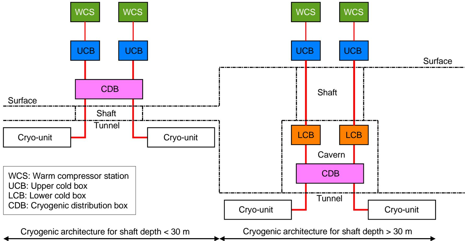
For shaft depth above 30 m, the hydrostatic head in the 2 K pumping line becomes prohibitive and active cryogenics (e.g. cold compressor system) has to be installed in caverns (LCB), i.e. additional cost for cryogenics and civil engineering.
