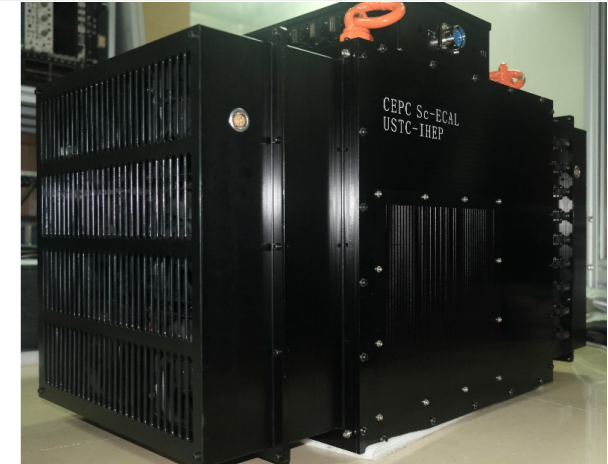
The fully-integrated Sc-ECAL prototype
