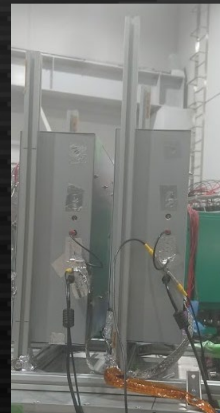
2 x testboards with sensor stacks inside the boxes set on the beam
