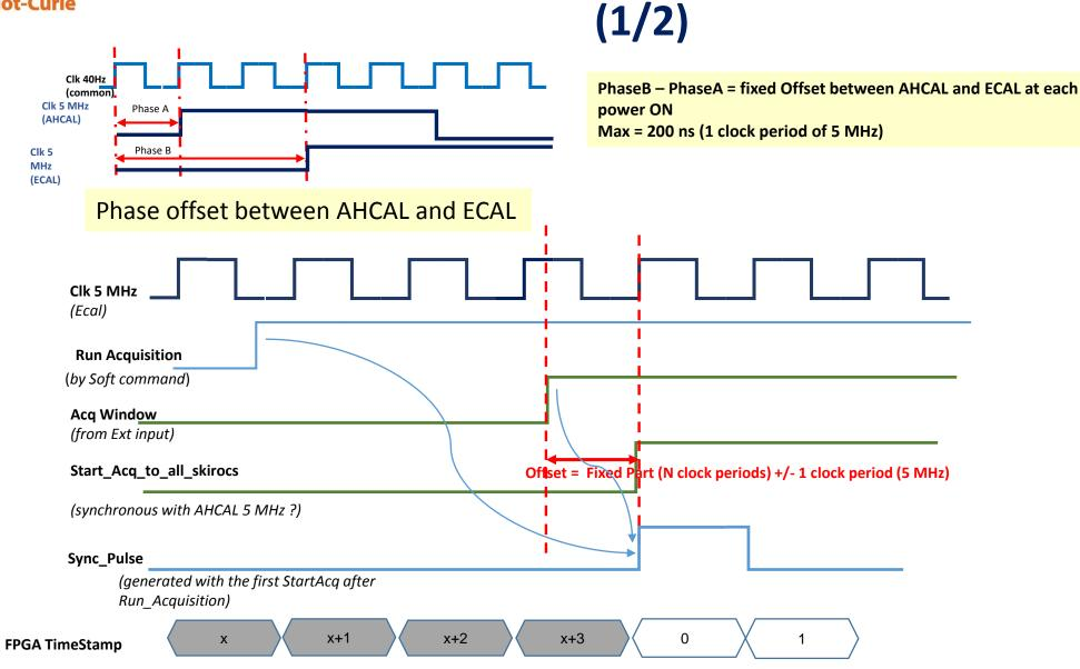
TimeStamps in AHCAL and ECAL have a **fixe offset part** due to synchronization stages in the firmware.
