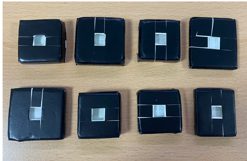
Glass tiles wrapped with Teflon and black tapes
