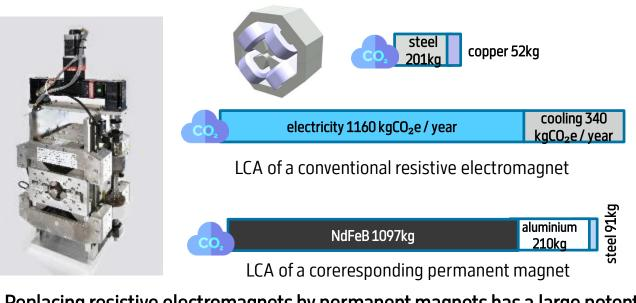
Replacing resistive electromagnets by permanent magnets has a large potential to reduce power consumption. The ZEPTO project has successfully produced ands tested tuneable permanent magnet quadrupoles. It is important to consider the full lifecycle to assess whether the savings are beneficial overall. Ref: B. Shepherd, ESSRI workshop 2022.
