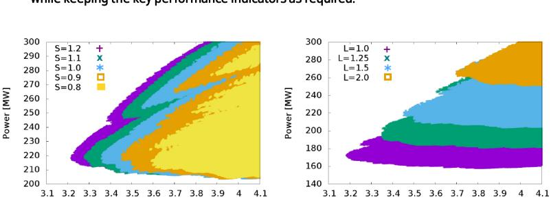
A scan of the CLIC parameter space was performed to find the optimal combination of parameters such as cavity gradient, iris, cells per structure, etc. Ref: arXiv:1608.07537, Sec. 3.3, and CLIC-Note-1031
