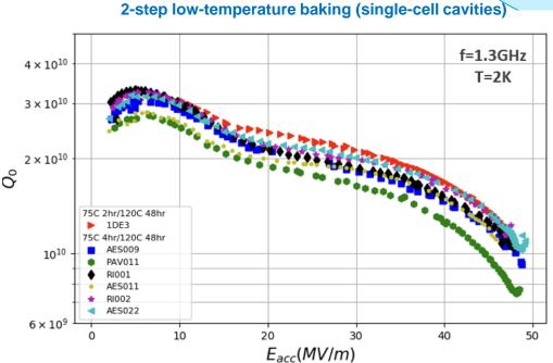
**R&D** pushes performance of superconducting cavities
