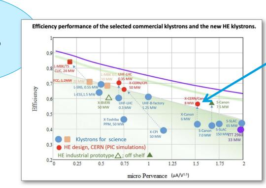
Development of high-efficiency klystrons based on novel beam optics (Core Stabilisation Method, Core Oscillation Method, Two Stage) greatly improves output power and efficiency of klystrons, reducing the energy demand of accelerators.
