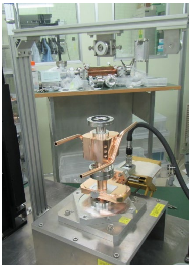
Figure 12: EBW of the quadrants. (a) After the EBW. (b) Welding penetration depth for the EBW conditions described in [13]. (c) A thermocouple is attached.
