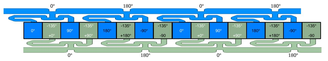
There has to be a phase difference of 135° between the upper and lower rf feeding manifold.
