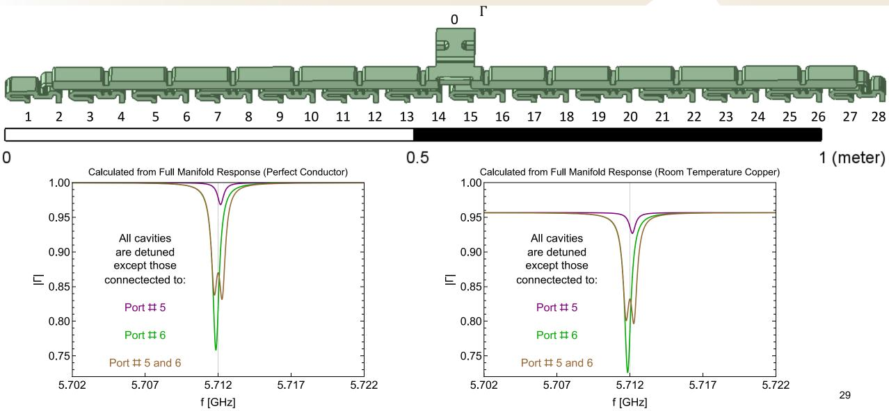
Each cavity is fed with rf signals of equal amplitude but phased advanced by  $-\phi$  with respect to the previous.
