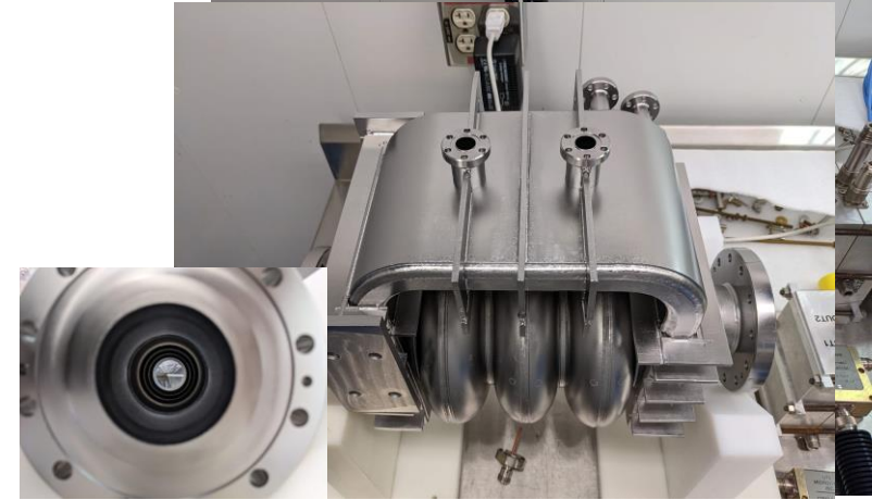
Cavity after 120um rotational BCP 800C bake, external BCP to remove oxides
