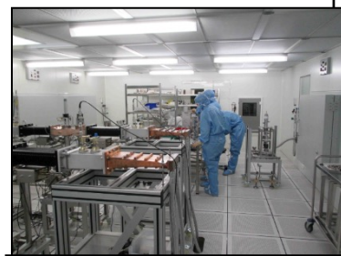
EU-XFEL : Preparation and power testing of 800 couplers
