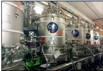
Spiral2 : Integration and test of 7 cryomodules
