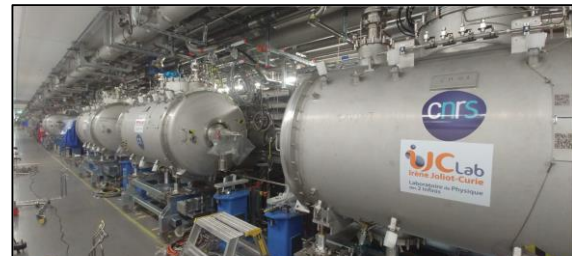
ESS : - preparation & testing of cavities, couplers and tuners - Integration of 14 cryomodules
