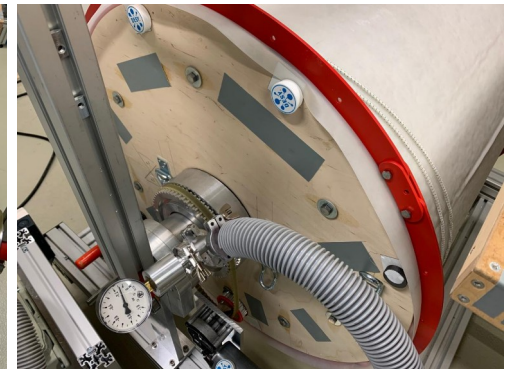
... put into vacuum bag \rightarrow pumping
