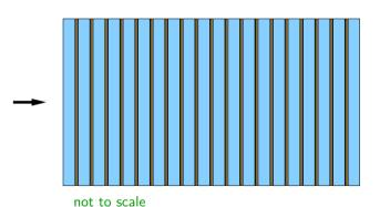
Best solution is always to instrument all calorimeter gaps.
