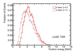
High rate of  $e^+e$  pair production expected due to non-linear effects (multi-photon scattering).
