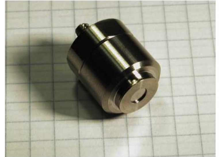
Fig. 3. The closed capsule (small design). The welding of the front ring is visible. The post has got a 6–32 UNC thread with a length of 6.3 mm.
