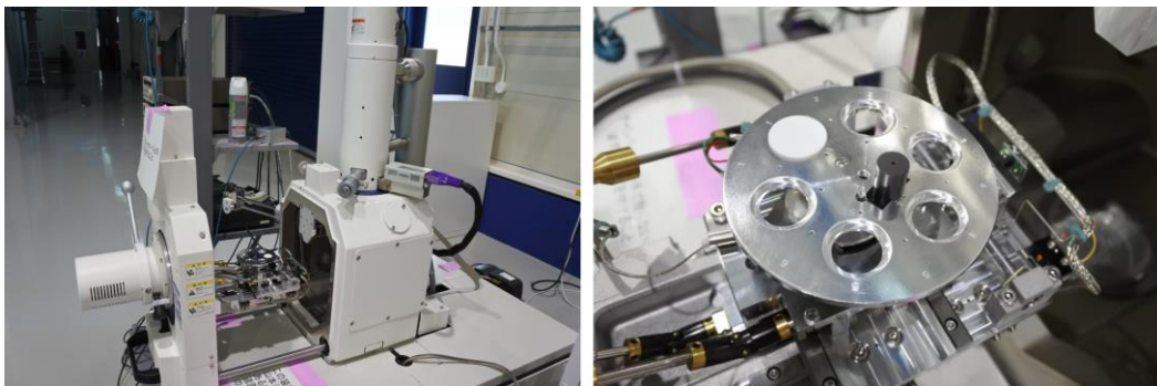
SEY measurement to check TiN coating
