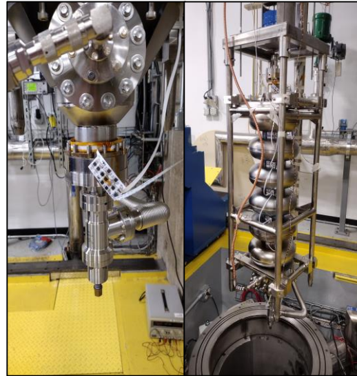
Figure 2: sXmap system mounted on HB60 SRF cavity
