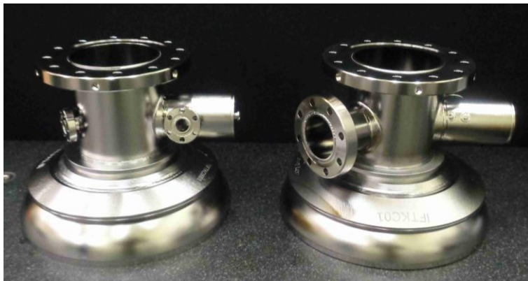
(End-cell + Beam-Tube) x2 EBW was done (24 Jan). Coupler-flange EBW was done (24 - 25 Jan).
