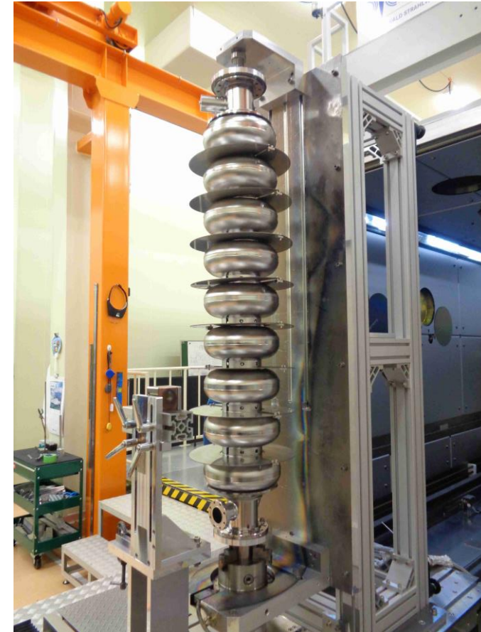
9-cell cavity assembly (31 Jan - 2 Feb): The equator-seam of cell x 5 was done.
