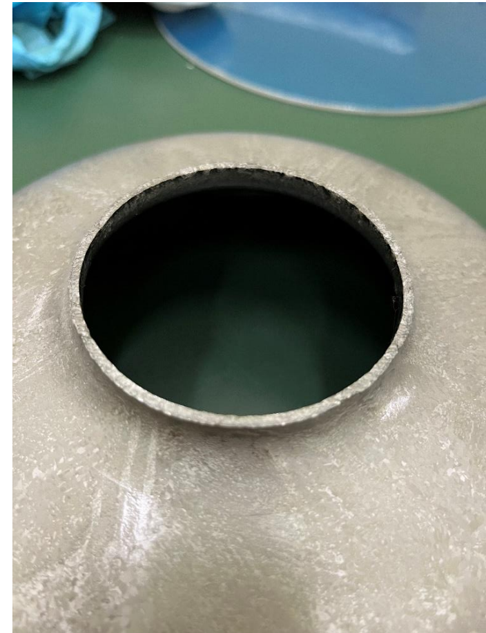
16 half-cells were press-formed.
