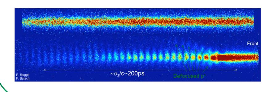
AWAKE has demonstrated that the selfmodulation of the proton bunch in plasma can be controlled [1,2], creating a train of microbunches suitable for acceleration [3].
