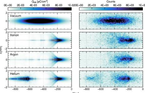
Top left: impact of ion motion on self-modulation in simulation and experiment [4].
