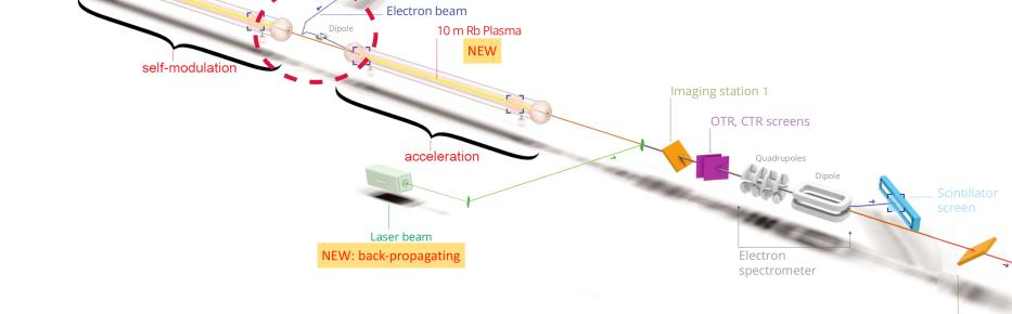
witness bunch will be injected into a second plasma for acceleration, allowing its emittance to be controlled during acceleration.
