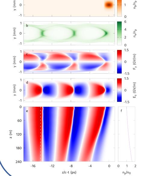
Above: the long train of microbunches can be harnessed to regenerate the wakefields, allowing the acceleration of multiple witness bunches [17].
