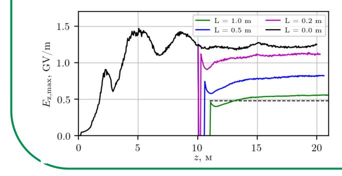
Left: The length of the gap between the self-modulation and acceleration stages modifies the the wakefields in the second plasma cell [8].
