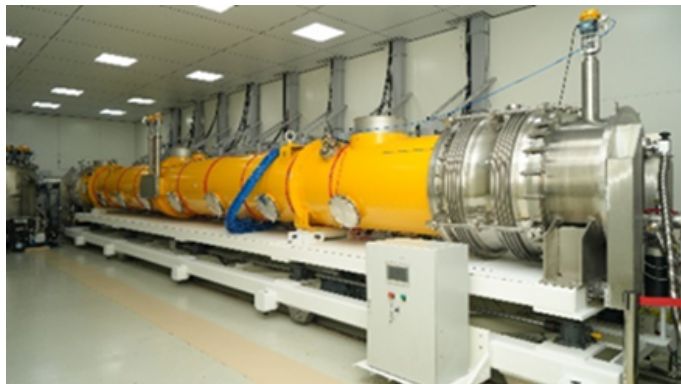
Figure 2. CEPC 1.3GHz full size cryomodule.
