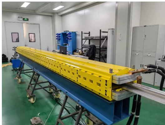
Figure 4. CEPC booster full size dipole magnet.
