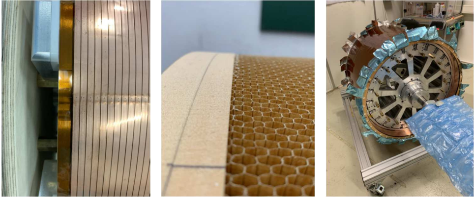
Fig. 11. a) Alignment of field strip foil. b) Routed flange honeycomb transition. c) Completed field cage being removed from the mandrel.
