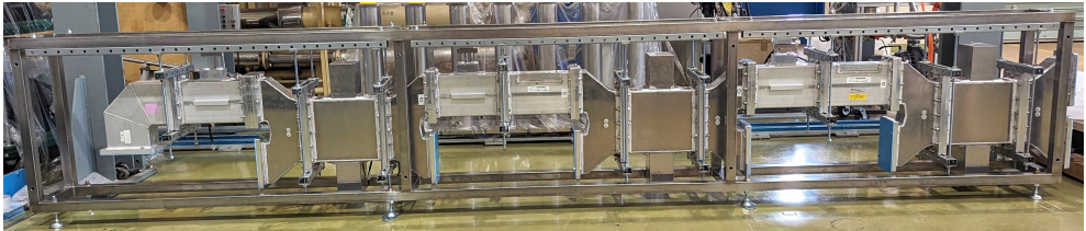
Figure 8. Integration of the sub-LPDS within the prototype support system.
