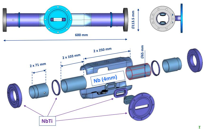
• All parts are milled from solid Nb ingots
