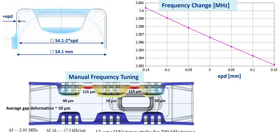
$\Delta f \sim -2.01 \text{ MHz}$   $\Delta f / \Delta L \sim -17.5 \text{ kHz/} \mu m$ vs. 10 kN force  $\Delta \sigma / \Delta F$  orce  $\sim 22 \text{ MPa/kN}$   $\sim 12 \mu m$  (1kN) tuner stroke for 200 kHz tuning
