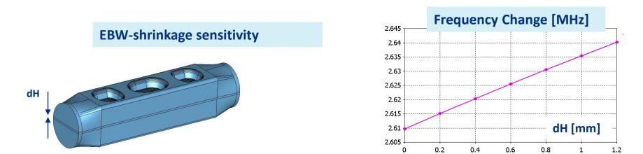
• Expected frequency sensitivity due to EBW shrinkage:
