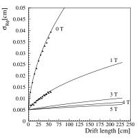
• Lines: Formula used in SGV:  $\sigma_{R\phi}^2 = \sigma_0^2 + (\beta_{slope} \sin \phi)^2 + \frac{D_{0T}^2}{1 + (\mu B)^2} \sin \theta Z$ ,  $\Rightarrow$  complicated relation, but gets better with shorter drift-length and higher *B*.
