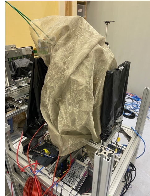
CDs are shielded by a metal mesh curtain
